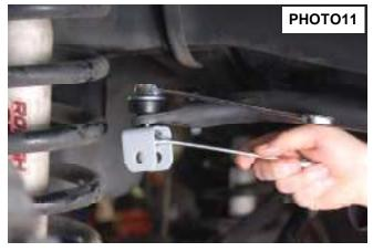
28. Install the supplied bushings / sleeves in the new sway bar links and install in the new sway bar bracket as shown **PHOTO 11** and on the factory axle location with supplied 12mm x 65mm hardware. **See PHOTO 12.** Tighten hardware.
