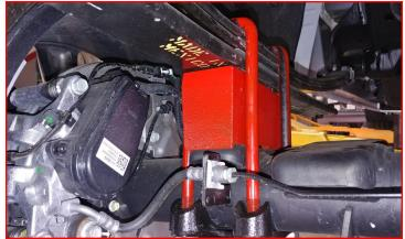
Install the shock extension using the provided M14 bolts, washers, and nuts to the top of the factory shock.
