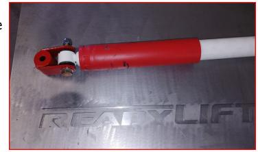
Install the ReadyLIFT shock extension to the frame using factory hardware
