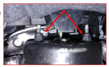
Remove upper control arm bolts located inside strut tower. Remove upper control arm from the vehicle at this time.
