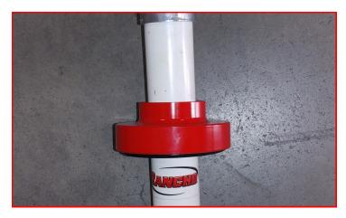
Ensure orientation of the strut assembly is as factory, install the shock. Using the spring compressor, Compress spring and install factory shock nut. Tighten and torque to 30-ft/lbs.
