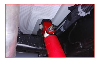
Remove factory bolt that attaches the rear jounce stop to frame and discard the bolt.
