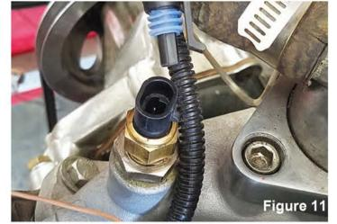
**Above** - The supplied Coolant Temperature Sensor is threaded into the water port in the intake manifold. Use Teflon tape on threads.
