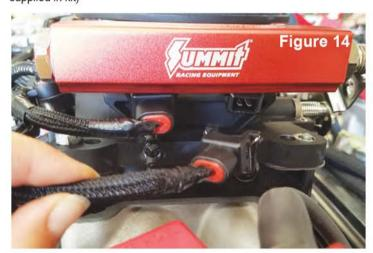
See Figure 7. Snap the connectors on the harness onto the individual injectors with the silver wire bar facing down. Make sure the connectors are securely fastened.
