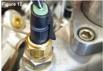
**Above** - The CTS connector on the main wiring harness is plugged into the Coolant Temperature Sensor in the manifold. (1/2" NPT adapter supplied in kit)
