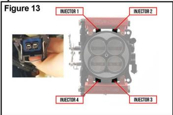
**Above -** The throttle body has four 66-lb injectors already installed. This arrangement will allow the system to supply enough fuel flow for up to 500 HP. The supplied Wiring Harness has four injector connectors.
