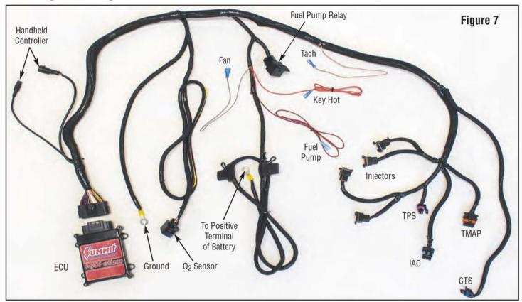
When installing the harness, the external ECU can be mounted anywhere in the engine bay or through the firewall. Be sure to keep it away from excessive heat. The harness is made up of the following connections: TMAP, IAC, O2, TPS, CTS, fan, tach, injectors, ground, positive connection to the battery, ECU, hand-held controller connection, fuel pump, and key hot.
