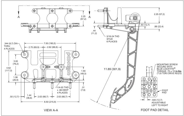
Reverse Mount Dual Pedal Assembly, Physical Dimensions (P/N 340-11299)
