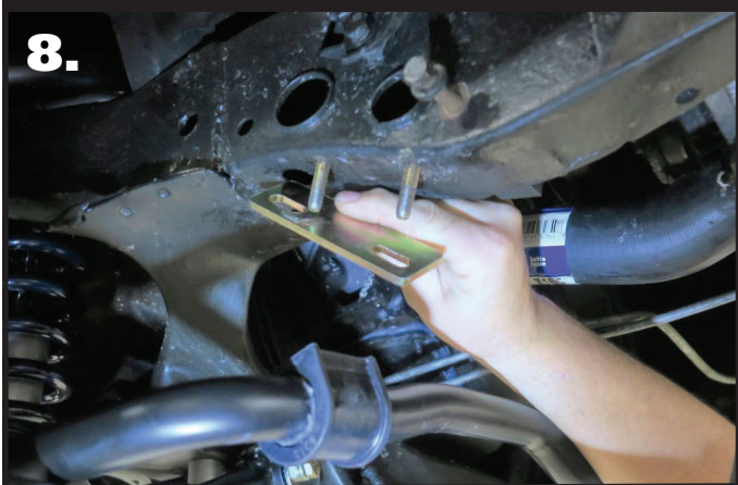
8. Install a 5/16" flat washer on each of (2) 5/16"-18 x 1 1/4" bolts and insert them into the OEM sway bar holes by inserting them in through the access holes in the side of the frame. Install the spacer plate with the wide side positioned to the inside. Hold it in place.
