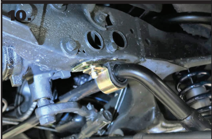
10. Lift the bar in position, the bolts sticking through the frame and spacer will go in the slots of the bushing strap. Hold the bar in place & install a 5/16" flat washer and 5/16"-18 nylok nut on the threads of each bolt sticking through the slots of the bushing strap. Repeat steps 8-10 on the opposite side, but do not tighten the hardware at this time.
