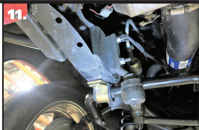
11. Reattach the idler arm to the frame using the OEM hardware. Torque the hardware.
