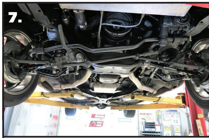
7. Insert the new swaybar from the passenger side. position it above the idler arm and steering arm. the center of the bar should hang down towards the ground.
