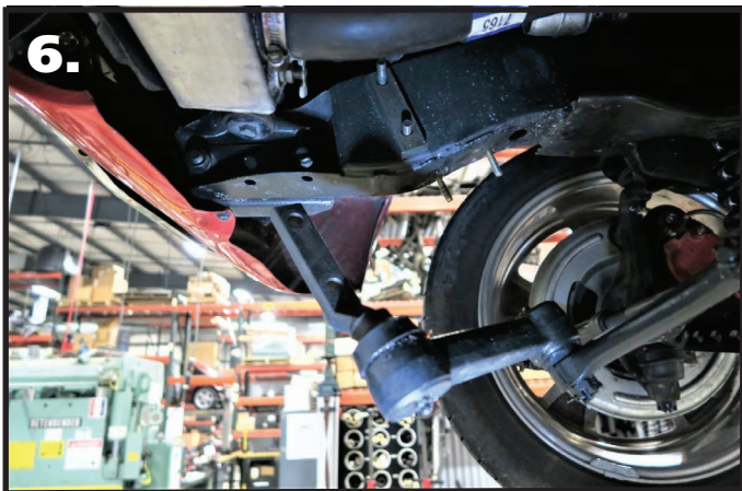
6. Disconnect the idler arms from the frame.
