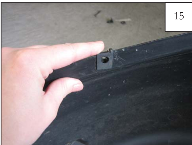
Install supplied #14 U-Clips over existing holes in splash shield (5 places). Flat side will be visible once splash shield is reinstalled.
