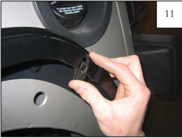
Install supplied Threaded Clips, with the thread side in, over holes in Inner Flare Piece (8 places).
