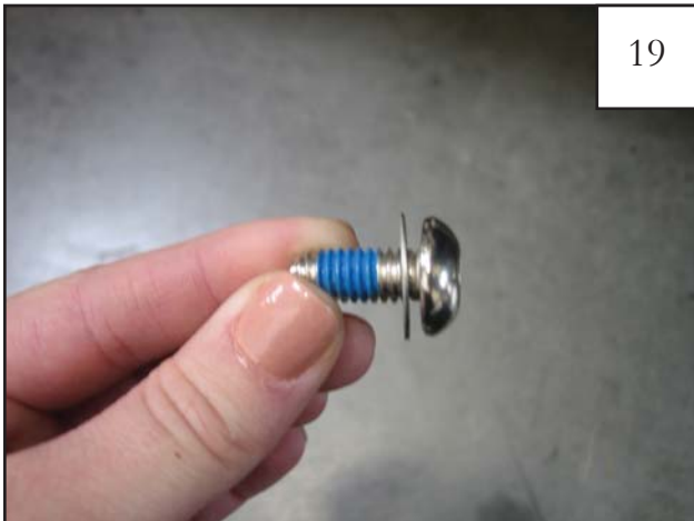
19 Position Rear Flare over Inner Flare Piece. Slide a supplied .700" Washer onto a supplied Torx Screw.
