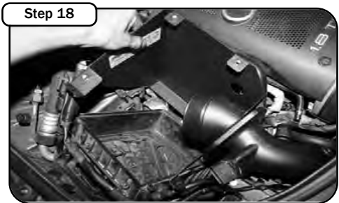
Step 18 Place aFe housing and tube into vehicle. Align housing clip on base and align sides of housing to airbox.
