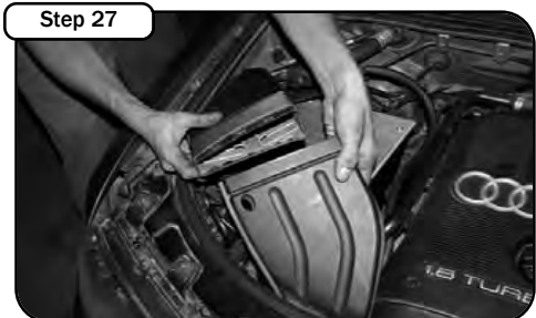
Step 27 Install factory fresh air duct and tighten down two screws securing it to the core support.
