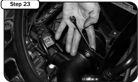
Step 23 Align tube to housing and use provided M6x1x25 screw, M6 flat washer, M6 wavy washer, and M6 nut.
