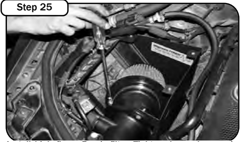
Step 25 Install high flow aFe air filter. Tighten down clamp using 5/16" Nut driver
