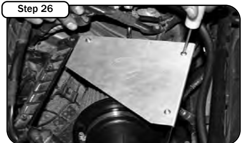
Step 26 Install aFe cover using (3) M6x1x10 button head screws.
