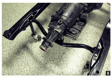
4. Re-install engine/trans (use of new engine mounts is recommended). With alignment/fitment of transmission determined, securely tighten CPP crossmember hardware (photo 5).
