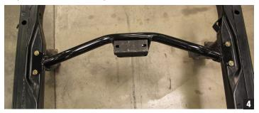
3. Install supplied 9425 transmission mount onto you 700-R4's tailshaft using the M10-1.5x25mm hardware.
