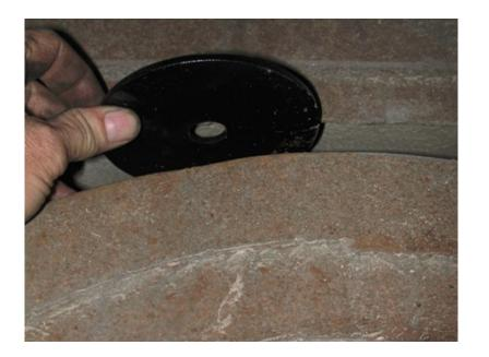
5. Place the 4.5" diameter washer on top of the coil spring pocket, between the frame and the body.
