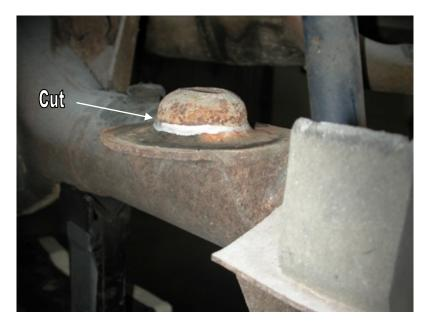
3. To allow the air spring to sit flat on top of the axle mount, the coil spring retainer must be cut down to about  $\frac{1}{4}$ " tall. Leave just enough of this retainer to locate the air spring roll plate, but make sure it is short enough not to contact the air spring piston.
