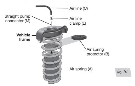
6. Attach the straight pump connector (M) to the air line (Fig. 10). Attach the straight pump connector to the air spring fitting. Do not use any tools to tighten the fitting.
