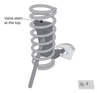
5. When the air spring is completely within the coil, remove the cap and allow the air spring to assume its "as-molded shape." Push the cylinder down to the bottom of the coil spring so that the stem at the top can be accessed for attaching the hose.
