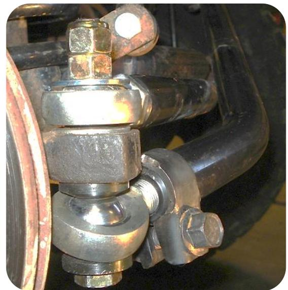
21. Install drag link at pitman arm using the following procedure:
