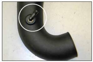
21. Install the 90° npt fitting into the  $K\&N^{\otimes}$  intake tube as shown.
