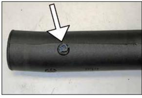
20. Install the inlet air temperature sensor into the  $K\&N^{\circledast}$  intake tube.
