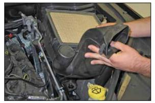
9. Lift up the lower airbox to dislodge it from the mounting grommets and then remove the lower airbox from the vehicle. Some vehicles may have a power steering line attached to the air box than will need to be unhooked.
