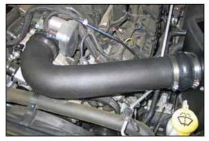
21. Install the K&N<sup>®</sup> intake tube into the hump hose at the filter adapter and then into the hose at the throttle body. Adjust the tube and heat shield for best fit and clearance and then secure with the provided hose clamps
