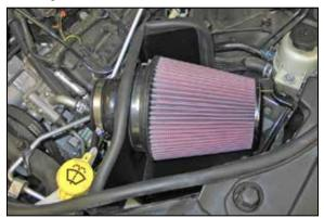
16. Install the K&N<sup>®</sup> filter onto the adapter and secure with the provided hose clamp. NOTE: Drycharger<sup>®</sup> air filter wrap; part # RF-1041DK is available to purchase separately. To learn more about Drycharger<sup>®</sup> filter wraps or look up color availability please visit http://www.knfilters.com<sup>®</sup>.
