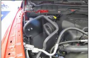
11. Reinstall the engine cover and route the crank case vent hose through the factory opening.
