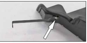
18. Install the heat shield mounting bracket (083103-1) onto the heat shield using the provided hardware.
