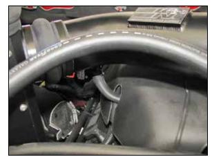
28. Connect the crank case vent hose to the fitting installed into the K&N<sup>®</sup> intake tube and secure with the provided hose clamp.
