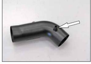
24. Install the vent fitting into the  $K\&N^{\ensuremath{\$}}$  intake tube as shown.
