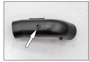
23. Install the provided grommet into the K&N $^{\mbox{\scriptsize \$}}$  intake tube as shown.
