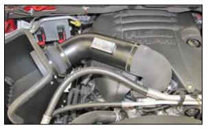
27. Install the K&N<sup>®</sup> intake tube into the silicone hump hose and then align with the hose on the throttle body. Align the hose, tube and heat shield for proper fit and then secure with the provided hardware.
