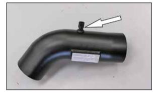
26. Install the inlet air temperature sensor into the grommet installed into the K&N $^{\odot}$  intake tube as shown.
