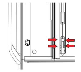
8 Using an awl, hammer and safety glasses, tap small divots at the marked locations. The screws are self-tapping and require a steady starting point.
