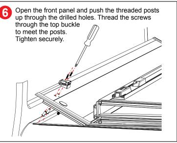
The cleat & strap and the bottom buckle will align straight with the mounted top buckle.
