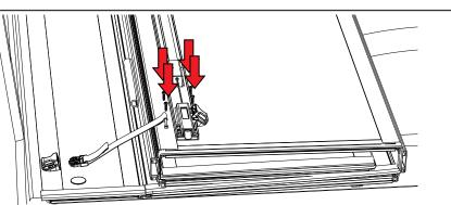
9 Mount the cleat and under buckle by driving the self-tapping screws through the cleat and buckle into the marked locations in each aluminum strip. The screws should be tightened securely, do not over tighten.
