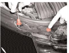
STEP 1 Open hood & remove the 4-Hex head screws fro the to of the stock grille. Then push down them pull out & up to remove the stock grille.
