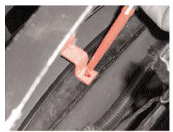
**STEP 4** Mount Billet Grille using factory screws from top of grille. Then mark the location that the bottom bracket sits on the steel bumper box. After you mark the location of bracket remove grille and remove the bracket from the billet grille.
