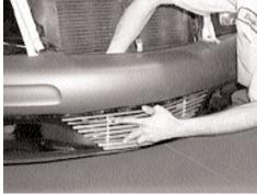
**STEP 2** Mount the lower grille at this point. If you don't it will be hard to get to after the upper grille is installed.
