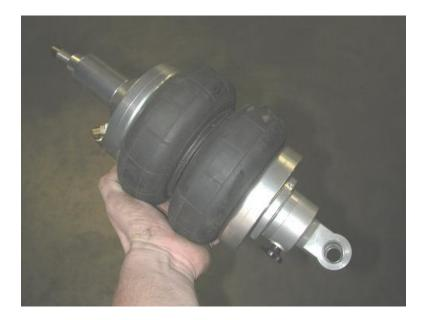
6. You will most likely have to drill the upper shock mount hole in the frame to <sup>3</sup>⁄<sub>4</sub>" to fit the Delrin ball setup. Assemble the Delrin ball setup according to the drawing on the next page. Raise the Shockwave up into the coil spring pocket with the Delrin ball stud top sticking through the factory shock mount hole. Secure with a 9/16" Nylok Jam nut.
