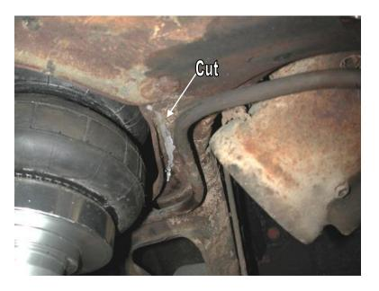
4. Here is another picture of the trimming that must be done.Make sure that there is sufficient clearance between the bellow and the frame through full suspension travel.
