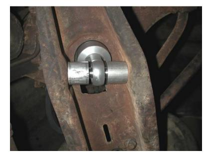
Bolt the Shockwave to the lower arm using a  $\frac{1}{2}$  x 4  $\frac{1}{4}$  bolt and Nylok nut. An aluminum spacer must be installed on each side of the Shockwave.
