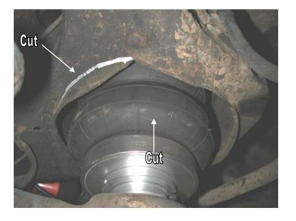
3. To allow for proper Shockwave clearance, so trimming must be done the lip around the coil spring pocket. This can be done with a die grinder and cut off wheel.
