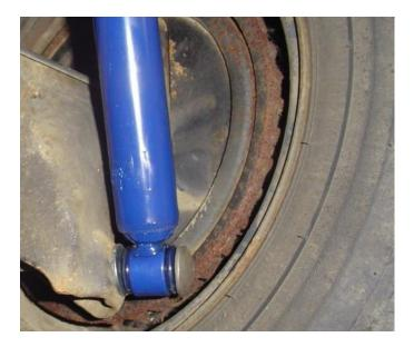
2. Attach the shock to the axle using the new cantilever pin supplied.
