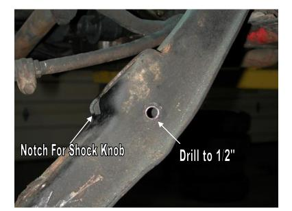
7. The lower shock mount hole will be used to mount the Shockwave. This hole must be drilled out to  $\frac{1}{2}$ ".
