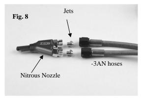
\*Note: Ensure that the fuel connection on the Nitrous Management Unit is connected to the fuel jet fitting on the nitrous nozzle. Ensure the same for the nitrous connections.
