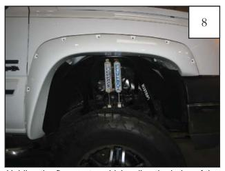
Holding the flare up to vehicle, align the holes of the flare with the factory holes in the wheel well.
