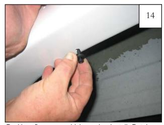
Position flare on vehicle and reinstall Retainers (RV1-P001).
