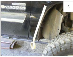
Starting at the bottom inside of the fender, cut through the inner and outer portion of the fender using a cutoff wheel and taking care not to cut into the bottom corner of the cab (behind the 1/4" foam insulation pad.
