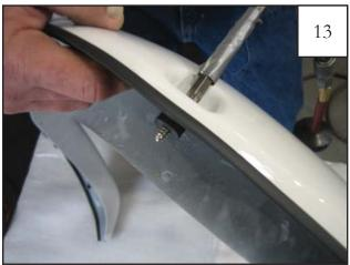
Using the supplied Torx Bit (SW1-0052), tighten the Spacer so the end of the Screw is visible.
