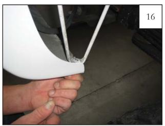
Reinstall factory support rod bolts through the 3/8" holes in flare and secure, making sure not to overtighten and crush flare.
