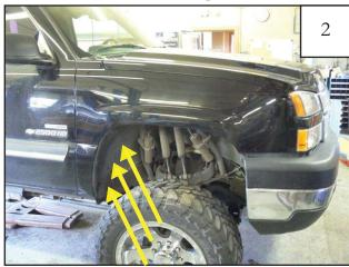
Remove three fasteners from the inner splash shield. Save fasteners for reinstallation.
