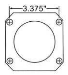
This kit is for axles with a 3 3/8" spread center to center on the top two bolt holes (pictured left). If your axle flange measures 3 1/8" from center to center, you need our AFXRD01, AFXRD05, AFXRD06 or AFXRD07.Call 800.405.2000 for further assistance.
