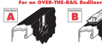
For each clamp mark on your bedliner a  $1-1/2" \times 3"$ hole as shown above. Remove clamp. Cut holes in bedliner. Reinsert side rail clamp. Return to step 6.
