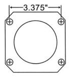
This kit is for axle with a 3 3/8" spread center to center on the top two bolt holes (pictured left). If your axle flange measures 3 1/8" from center to center, you need our kit AFXRD01 or AFXRD05.
