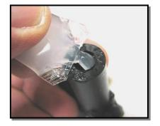
Insert the terminal/wire into the boot and check for proper alignment. Make sure that the open end of the terminal is visible when looking down into the boot.
