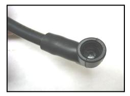
NOTE: The ThunderVolt wire will measure approximately 40 ohms / foot (+ or -20%) resistance. Due to the sophisticated conductive nature of this core, it will require you run the engine for a minimum of 2 minutes, then immediately measure the resistance in order to get an accurate measurement.
