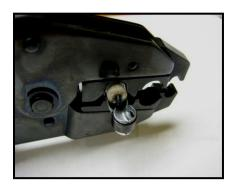
Form the tabs of the terminal to hold everything in place for crimping. Crimp the terminal with a Taylor #43400 or #43390 crimp tool or other appropriate crimp tool.
