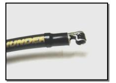
Put some of the silicone grease on the terminal, heat shrink tubing, and inside the boot as this will aid in the installation of the distributor boot.
