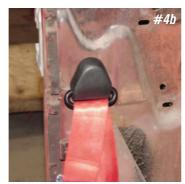
**Photo #4a & 4b:** The upper seat belt slide has a 7/16" X 1" bolt that passes through the inner quarter panel and bolts solid to the 1" X 2" bracket. Tighten the bolt and install the plastic cover. The cover can be painted to match the interior if so desired.
