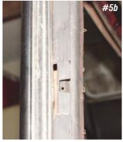
**Photo #5a & 5b:** On a 2-door sedan, wagon or Nomad, there is a slot in the forward quarter glass body channel metal. To access the channel, the vertical fuzzy channel must be temporarily removed. The upper seat belt anchor bracket can be fed through the slot in the body. Drill a 1/2" hole 5" up from the base of the quarter window for the anchor bolt and upper belt mounting point. The bolt will thread into the bracket that is trapped in the body.
