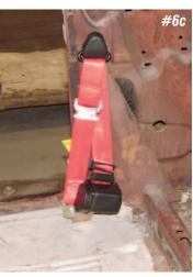
**Photo #6a, 6b & 6c:** The seat belt retractor and the end of the seat belt are held to the floor bracket with a 7/16" X 1" bolt with two flat washers and a lock nut. Mount the retractor to the rear hole on the bracket and the end of the seat belt to the forward hole.
