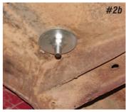
Photo #2a & 2b: The 7/16" bolt and small flat washer pass through the bracket and floorboard. Install the large flat washer and lock nut on the bottom side of the floor and tighten.
