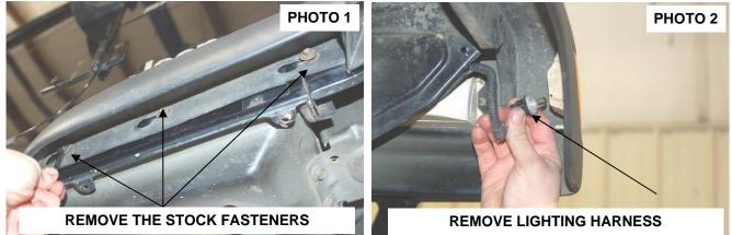
3. Remove all he stock flare hardware using a 8mm wrench. Remove the flare from the vehicle. See Photo 3.
