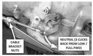
A. Manually move the selector lever to the NEUTRAL detent (3 clicks back from LOW / full-forward), and move the shifter to the NEUTRAL position. Adjust the cable bracket nuts (and the swivel, if necessary) until the swivel slips freely in and out of the selector lever hole.
