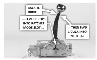
A. On the transmission, manually move the selector lever to the NEUTRAL detent (that is, 2 clicks back from full-forward / PARK). Then in the vehicle, move the shifter first to the DRIVE position (4 clicks back from full-forward, when the shift lever drops into the ratchet mode slot), then push it forward into NEUTRAL.
