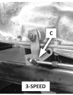
B. Adjust the cable bracket nuts (and the swivel, if necessary) until the swivel slips freely in and out of the correct hole in the selector lever ("F" for 4-speeds; "C" for 3-speeds). Gradually tighten the cable nuts against the bracket, while continuing to check the fit of the swivel in the selector lever.
