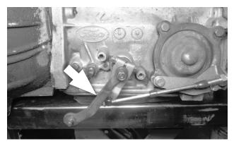
**35.** Reinstall the throttle lever, lock washer and nut on the throttle shaft and tighten securely. The throttle lever must operate smoothly with no binding.
