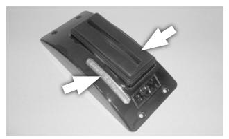
57. Install the shifter boot and the appropriate indicator window in the tower cover. (Use the 4-speed window for GM 4-speed transmissions only; use the 3-speed window for all others, including 4-speed Chryslers and Fords.)
