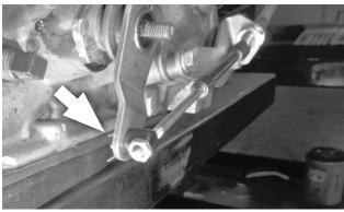
**34.** Secure the swivel to the selector lever with the cotter pin. Operate the shifter through all the gear positions, verifying that it operates correctly.
