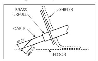
**CAUTION:** Do not kink the cable anywhere along its length, or it will lock up. The cable should be kept straight for at least 2" after it leaves the brass ferrule at each end.
