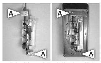
**58. Verify the shifter mechanism is free of any debris** and loose hardware. Remove the shift knob, and place the tower over the shifter. Align the tower's through-holes with the outboard screw holes on the shifter's front and rear brackets (at locations "A").
