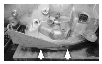
14. Install the cable bracket at the two pan bolt holes directly below the selector lever, using the two 5/16-18 × 1" bolts and flat washers. For stamped sheet-metal (stock) pans, use the two spacers between the pan and bracket. (Spacers are not used with cast aluminum pans.) Tighten the bolts to 12-13 ft-lbs torque.
