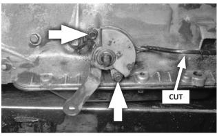
26. If your transmission is equipped with a neutral safety / backup light switch: Remove the two mount bolts and slide the switch off the selector shaft. Cut the wiring harness between the switch and its connector, and discard the switch. (The wires from the connector will be routed to the B&M switches later.)
