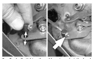
B. Gradually tighten the cable nuts against the bracket while continuing to check the fit of the swivel in the selector lever. Then with the swivel inserted in the selector lever, lightly snug the jam nut.
