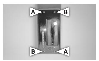
**59.** Place the assembled cover over the shift lever and tower. Hand-start two of the **10-32** × **3/4**" self-tapping screws at hole locations "A" (through the tower, into the shifter's outboard screw holes). Then carefully start the other two
