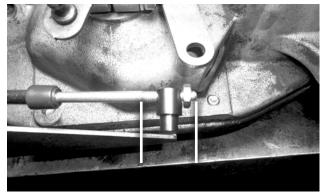
**16.** Thread the swivel onto the cable to about the middle of the threaded section, then reinstall (but do not yet tighten) the jam nut.
