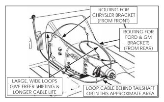
10. Route the cable approximately as shown, based on your application. Avoid any sharp bends which may kink or otherwise damage the cable. Seal the cable hole shut
