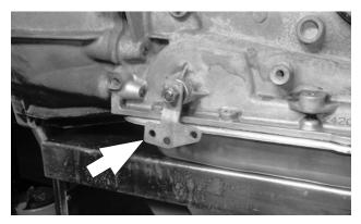
**41. Install the B&M selector lever** using the stock selector lever nut, and tighten the nut to 23 ft-lbs torque. The lever should travel smoothly back and forth, with a positive "click" in each detent.
