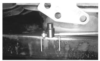
**45.** Thread the swivel onto the cable to about the middle of the threaded section, then reinstall (but do not yet tighten) the jam nut.
