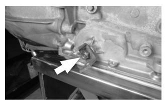
**40. Disconnect stock controls:** Remove and retain the selector lever nut. Remove and discard the selector lever and shift linkage.
