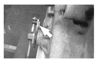
**48.** Secure the swivel to the selector lever with the cotter pin. Operate the shifter through all the gear positions, verifying that it operates correctly.
