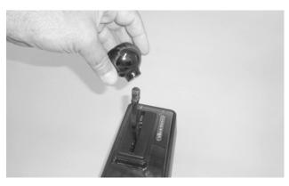
**60. Apply medium strength thread locker** to the shift lever threads. Carefully thread the **shift knob** all the way onto the lever and hand-tighten.
