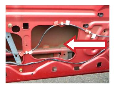
**STEP 1a:** Install the window regulator through the main access hole.
