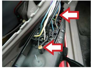
**STEP 3:** Using a Phillips head screw driver, remove the master power switch assembly.
