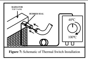
4. Connect the pump wiring harness to the pump. Cut the blue wire before the fuse and crimp the spade terminals (from Thermal Switch packaging) to each end. Connect spade terminals to each pin of thermal switch. The connection order does not matter since both pins have the same polarity. The blue wire provided with the thermal switch can also be used to increase length of blue wire form EBP<sup>®</sup>, otherwise this can be discarded.
