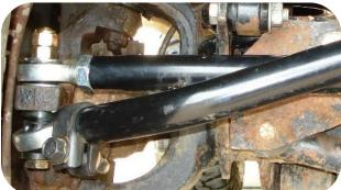
For 33-36" tire diameter (measured): adjust your tie rod until the front measurement is 1/8" less than your rear measurement. Adjustment can be done by removing only the driver's side bolt and you can turn the whole tie rod if needed to adjust both sides equally.
