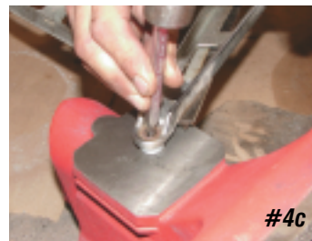
Photo #4a & 4b & 4c & 4c & 4d & 4e: With the roller and rivet in place, first use a tapered punch and flare out the tube end of the rivet. Next using a flat punch, smash the edges of the tube rivet down tight on the window frame. This will center and tighten the rivet in the hole on the window frame or regulator.
