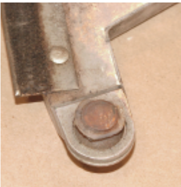
Photo #1: Here is a photo with normal wear on the original nylon roller.
