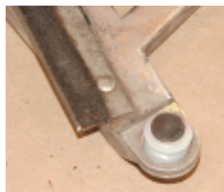
Photo #4a & 4b & 4c & 4c & 4d & 4e: With the roller and rivet in place, first use a tapered punch and flare out the tube end of the rivet. Next using a flat punch, smash the edges of the tube rivet down tight on the window frame. This will center and tighten the rivet in the hole on the window frame or regulator.
