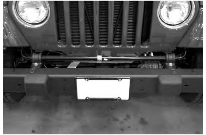
Figure #8 – Factory Front Panel Removed
