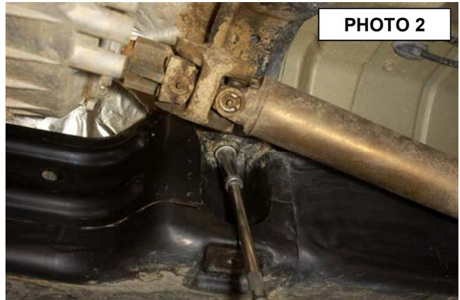
3. Remove the bolt from the inside of the of the gas tank pocket 18mm and remove the factory skid plate.
