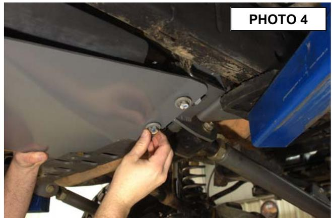
5. Insert the stock bolt on the frame side of the skid plate and tighten with a 18mm socket. See **Photo 5**.
