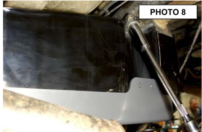
9. Locate the correct mounting bracket and insert factory bolt in the top of the bracket. Hand tighten. Use two of the supplied 7/16" x 1" bolts and washers to attach the skid plate to the bracket. Tighten with a 5/8" socket. Tighten the factory bolt holding the bracket with a 18mm socket. **See Photo 9.**
