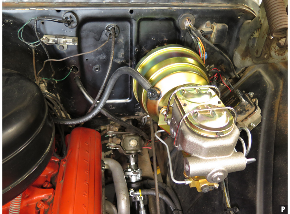
13. Shown with #5559FBB2 master cylinder and booster assembly installed. (Fig P)
