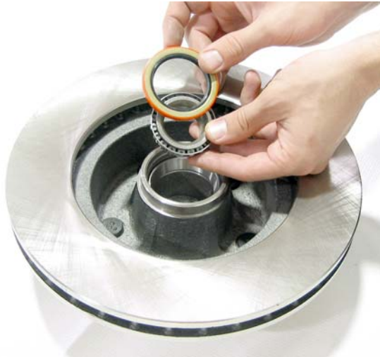
Inner Bearing Assembly
