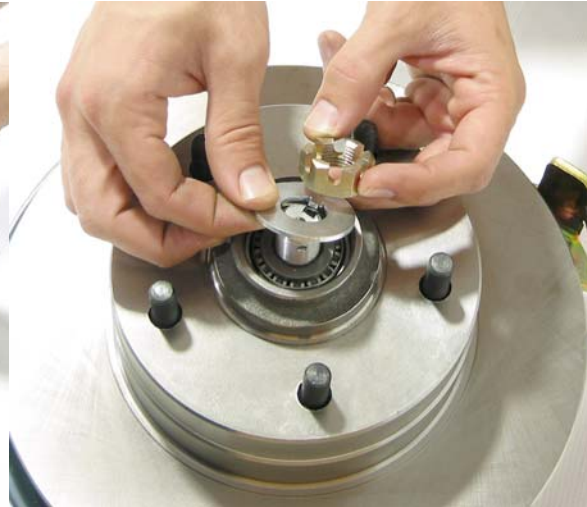
Outer Bearing Assembly
