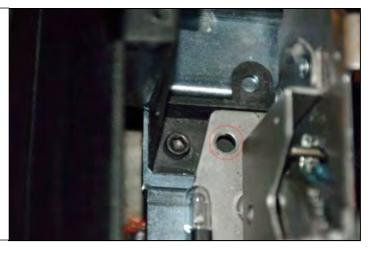
24. Re-install console. Secure the center of the console to the bracket with two (2) of the 1/4"-20 socket head cap screws provided in the hardware kit. Re-use the original screws to secure the front and rear of the console.
