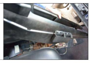
11. Remove shifter cable retaining clip.
