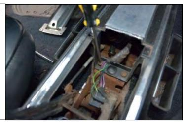
6. Remove the two (2) screws that are securing the front end of the console to the floor.
