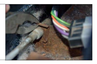
12. Remove the retaining clip that is securing the end of the shifter cable to the shifter. Then remove the cable from the shifter.
