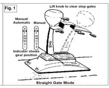
**Park:** To get to park from any straight gate position, lift the handle all the way up and push forward. The transmission will find its own Park position. Release the handle and the shifter is locked in Park. To get any other gear position, you must raise the shifter handle to clear the stop gate.
