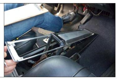
5. Remove the two (2) screws that are securing the center of the console to the shifter.
