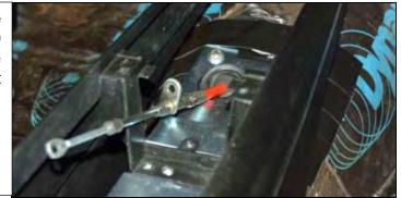
25. Install shifter. Secure the shifter to the bracket with four (4) of the 1/4"-20 socket head cap screws provided in the hardware kit. A spacer has also been provided to add support between the upper left mounting point of the shifter to the bracket. If the console is OEM then it might require further modification to utilize the spacer.
