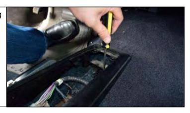
7. Remove the two (2) screws that are securing the rear of the console to the rear bracket mounted to the floor. You must open the compartment door to access screws.
