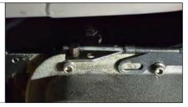
18. Remove the two transmission oil pan bolts from the middle of the left side of the oil pan. Install the cable bracket in position. The bracket must be installed with spacers between the pan and the bracket. Install two 5/16 x1.00" bolts (or M8 x 25 mm for metric transmissions) supplied and tighten 12-13 ft. lbs. Do not overtighten as this can damage the pan gasket.
