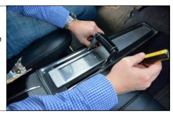
3. Lift the shift indicator assembly from the console, unplug the two (2) bulb harnesses from the shift indicator assembly and set aside.
