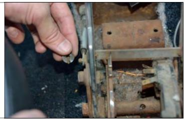
13. Remove the four (4) screws that are securing the shifter to the floor. Remove the shifter.
