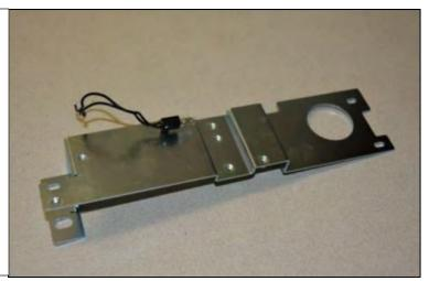
21. Install the bracket with the four (4) 1/4"-14 drilling screws and 1/4" washers.
