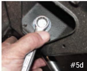
**If you are using stainless steel hardware, you must, must, must use anti-seizing compound or a thread lubricant specifically for stainless steel on the bolts. If you do not, you will gall the fasteners. The nut will permanently seize to the bolt!**
