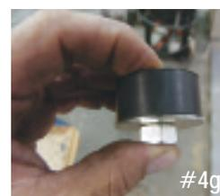
It's a good idea to use some ant-seize compound on carbon steel bolts when assembling them into the cushions. Using the
