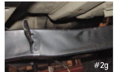
**Photo #2a, 2b, 2c, 2d, 2e, 2f & 2g:** With all of the body mount bolts cut, we're ready to jack up the body to gain adequate space between the frame and the body to work. Using a piece of scrap lumber and your floor jack, begin to slowly separate the body from the frame (Photo 2a). This piece of wood will
