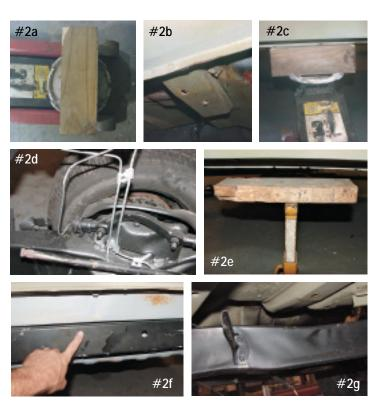
Photo #2a, 2b, 2c, 2d, 2e, 2f & 2g: With all of the body mount bolts cut, we're ready to jack up the body to gain adequate space between the frame and the body to work. Using a piece of scrap lumber and your floor jack, begin to slowly separate the body from the frame (Photo 2a). This piece of wood will
