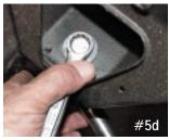
1A). Your assembled mount should look like this on the car (Photo 5b). Adjust the torque wrench to 40-50 foot-pound torque setting (Photo 5c). Lastly, using your 5/8" hand wrench and a deep well socket on your torque wrench, torque the nut while holding the bolt (Photo 5d). Repeat this process on all other mounting points; they all go together in a similar fashion.
