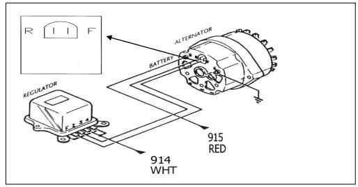
Figure 7-1 Early GM Alternator - External Regulator
