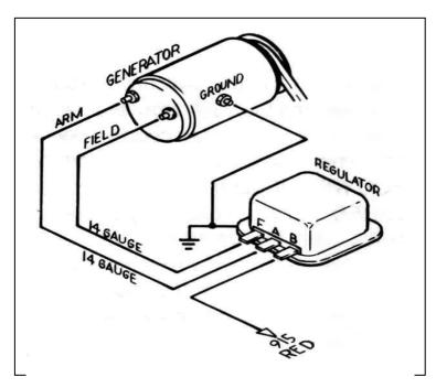
Figure 10-1 Generator Charging System
