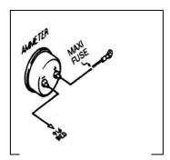
Figure 10-2 Ammeter & Maxi Fuse
