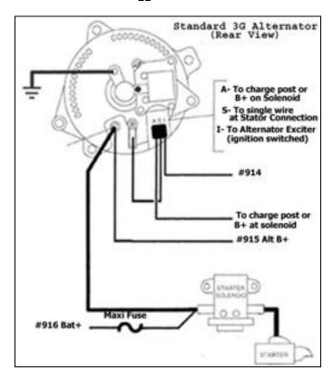
Figure 8-1D Ford 3G ALternator
