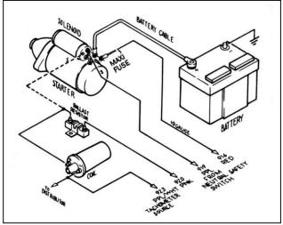
Figure 7-4 GM Ignition (Start-Run) System
