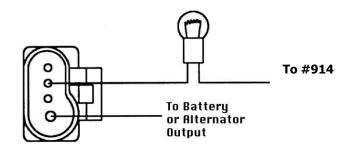
NOTE; If not using a charge light, an 82 ohm, 5 watt resistor must be used to prevent premature Regulator failure
