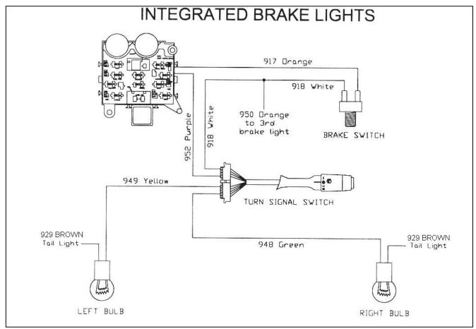
Figure 10-7A Integrated Brake Lights
