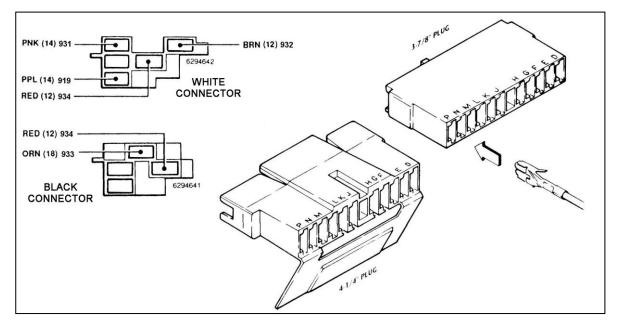
Figure 7-5 GM Turn Signal Connectors
