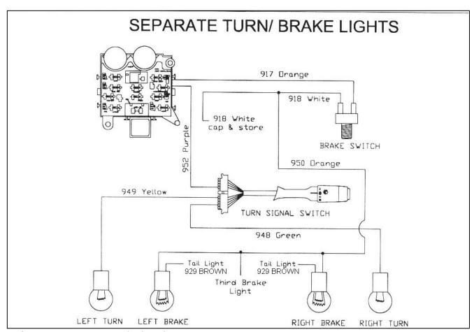
Figure 10-7B Separate Turn/Brake Lights
