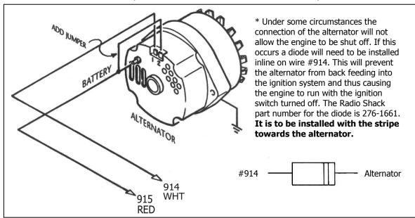
Figure 7-2A Late GM Alternator - Internal Regulator
