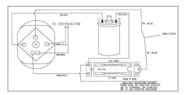
Figure 9-2B Mopar Electronic Ignition with Dual Ballast Resistor
