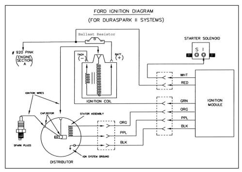
Figure 8-4 Ford Ignition Diagram (Duraspark II Systems)
