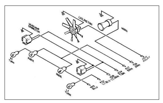
Figure 10-4C HEADLIGHT SECTION A Wiring
