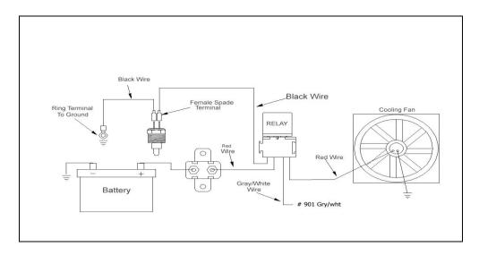
Figure 10-4B Typical Fan Relay with Thermostat (Painless Part # 30102)
