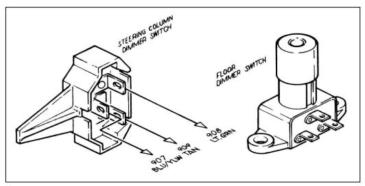
Figure 10-5 Dimmer Switches (Push Button Style - Painless Part #80150)
