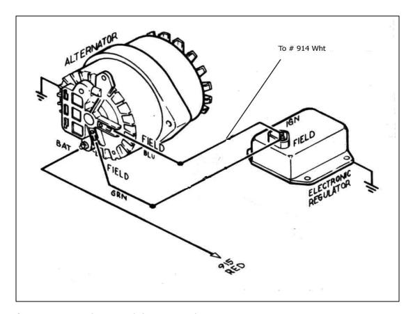
Figure 9-1 Mopar Alternator w/ Electronic Regulator
