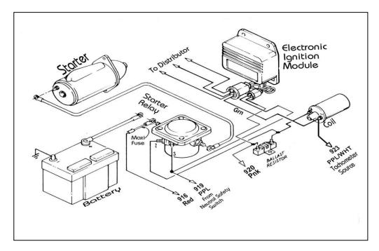
Figure 8.3 Motorcraft Electronic Ignition System
