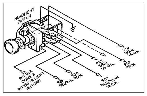
Figure 10-6 HEADLIGHT SECTION B Wiring (Painless Part #80152)
