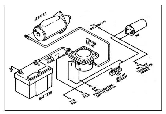
Figure 8-2 Ford Ignition (Start/Run) System
