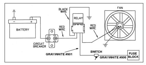
Figure 10-4A Typical Fan Relay Installation (Painless Part #30101)
