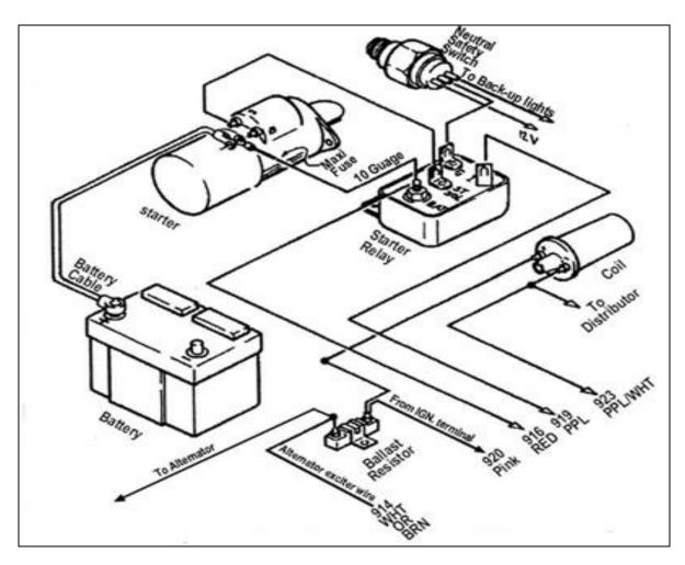
Figure 9-2A Mopar Ignition (Start/Run) System
