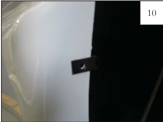
10 Install Clip (CL1-0011) over existing factory hole.
