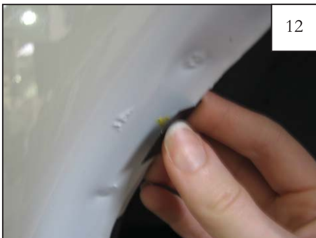
12 Install Tab (MT1-0014) on sheet metal centered over mark.
