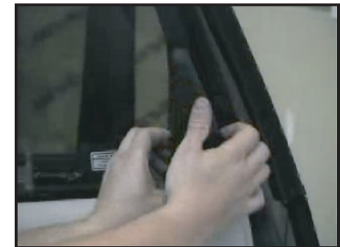
15. Next, remove reardoor panels: First, remove small window panel.
