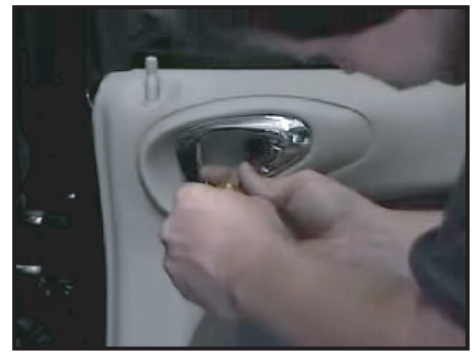
18. Remove screw from behind door release lever.
