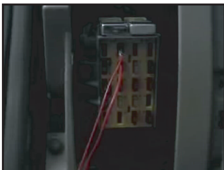
13. Connect the red wire to the constant 12v source. This source will have 12v at all times.
