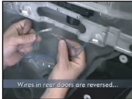
32. Wires for rear doors are reversed.
