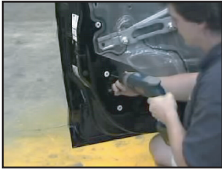
7. Mount front actuator; Drill top mounting hole...
