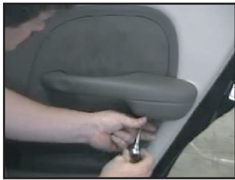
16. Remove Screw from bottom right of door handle.
