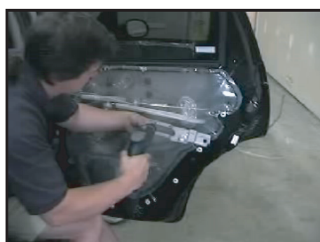
26. Mount rear actuator; Drill front hole...
