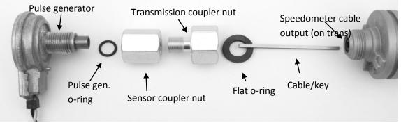
"Exploded" view of sensor install
