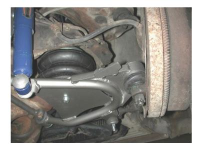
5. The air spring will be attached to the lower arm using a 3/8" x 3/4" bolt, lock washer and flat washer.
