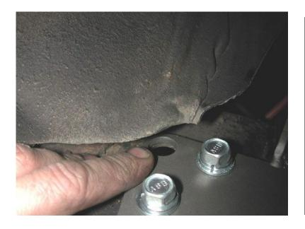
2. Mark the hole in the bottom of the frame and drill with 5/16" bit. Use the 3/8" self-tapping bolts supplied and bolt the bracket to the frame. Mark and drill the remaining holes.
