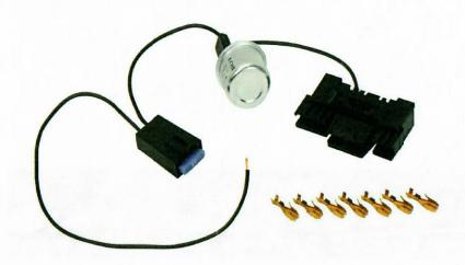
The Hazard Kit (FR20118-1) is the perfect fit for any owner looking to add hazard light (4-way flasher) functionality to their classic vehicle! The 4-1/4" female connector connects directly to the wiring harness on Flaming River's Tilt Columns. This kit includes one female connector, 12V flasher, 15A fuse, and seven spare crimp terminals to plug in additional wires to the provided connector.
