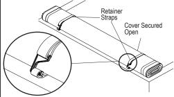
Secure cover open by hooking retainer straps to front loops.
