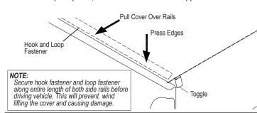
STEP 8: To open cover, pull rear release toggle. Start rolling cover toward cab making sure both sides of cover roll evenly. For best results, leave unrolled portion of cover attached to the hook and loop fasteners while opening.
