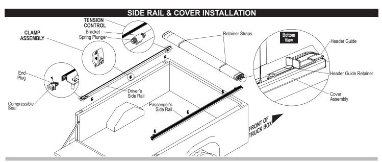
STEP 1: Attach the TruXedo rails to the truck's vertical inside flange as ISTEP 2: For optimum latching performance and cover fit, side rails shown in Detail A. To get the correct TruXedo rail alignment from front to back, See Detail-B. Compress the rear seal against the closed tailgate and hold. Attach clamps starting at the tailgate. Evenly space 3 clamps along each TruXedo rail,
