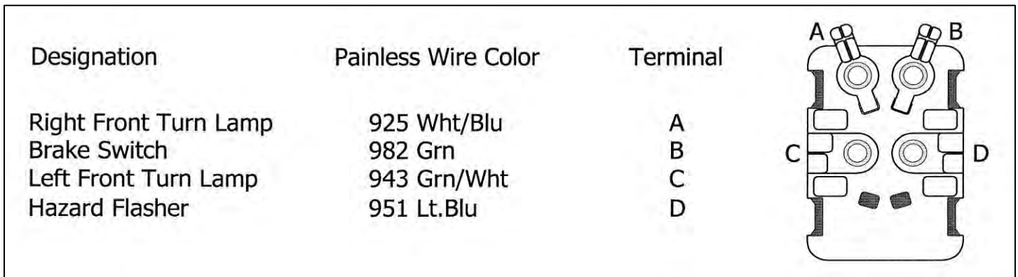
Figure 7-11 Hazard Switch Wiring
