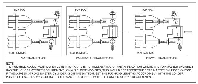
Figure 3. Push Rod Length Adjustment
