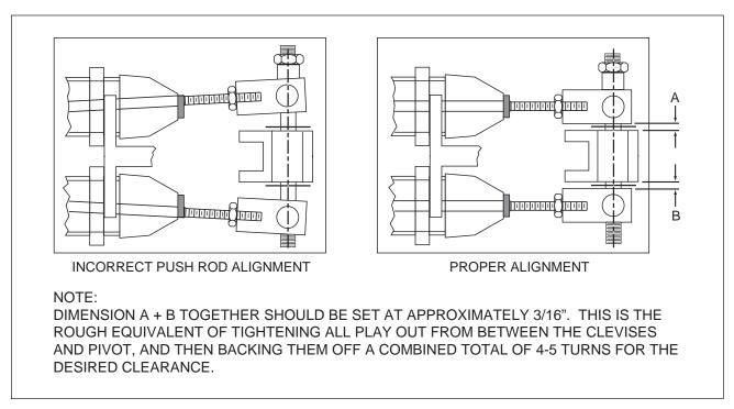
Figure 2. Push Rod Alignment
