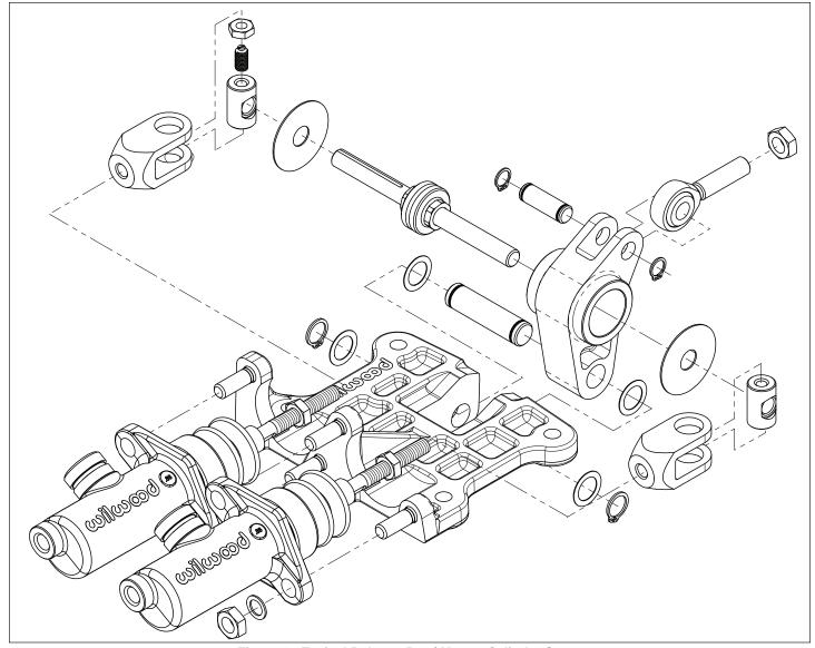
Figure 1. Typical Balance Bar / Master Cylinder Setup
