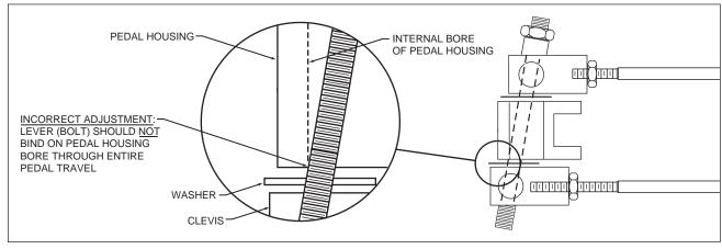
Figure 4. Balance Bar Lever Interference
