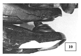
The white area of the lower control arm (**Photo 9 and 10**) indicates the interference area where wheel rim contact will occur when wheels with more than 3 ½" inches of backspacing are used. The installed lower control arm (top of pictures) has had its white area removed to provide clearance for non-recommended wheels. Please read entire caution under Step 11. **IMPORTANT NOTE:** <u>We do not recommend or approve this modification.</u>
