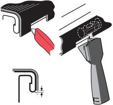
For bed liners that cover the metal flange, trim a minimum of 100 mm or 4" of the liner wall so the clamps contacts the bottom of the metal flange.
