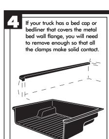
For bed caps, trim only enough of the bed cap edge so the rear (tailgate) clamp contacts the bottom of the metal flange.
