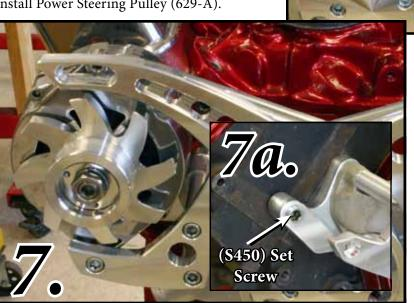
FIG 7. Install (S450) threaded bushing into alternator rear support bracket (as shown Fig 7a). Install the Alternators (P573) using (1)  $\frac{3}{8}$  x  $5\frac{1}{2}$ " SHCS (S280) and a TP3-1.775 Spacer Between the rear of the Alt and the (S450) Set Screw. Turn the S450 set screw to take up any slack between the lower alternator support and the spacer. Secure with a  $\frac{3}{8}$ " Lock Nut. (S622). (snug only at this time).
