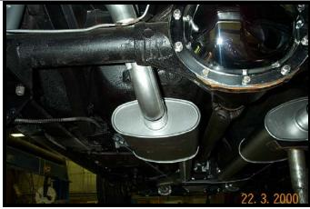
5) Mount the hanger brackets to the existing holes in the frame behind the rear axle using the lag screws and the snapper grommet (see drawing). The hangers should be installed to the tail pipes at where the tail pipes cross under the frame. Two additional hangers have been included to use at your preferred location.
