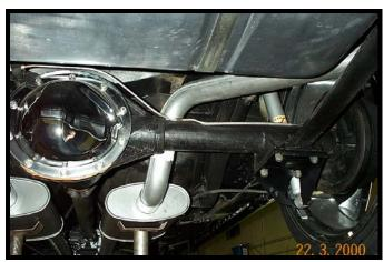
7) Make sure that all the parts of the system are clear of frame members, all hoses, suspension, and brake and fuel lines. Starting at the collector pipes, tighten all connections and nuts. Make sure all parts are clear and will not leak or rattle. After several days of driving retighten all bolts.
