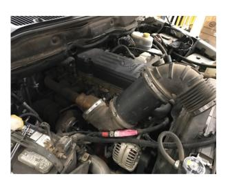
**STEP 5**Install the Tube Seal (C) onto the AirBox (A).
