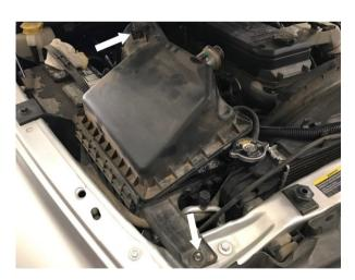
**STEP 4**Loosen the hose clamp at the turbo inlet and then
